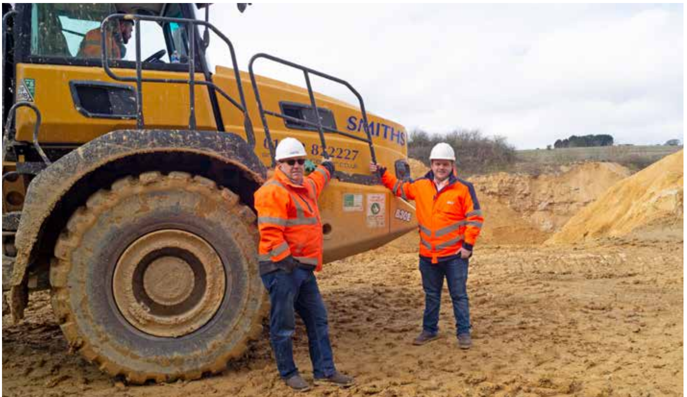
UK construction company, Smiths of Gloucester, worked on a contract that required a sustainable fuel solution for all plant and equipment and successfully ran two Bell B30Es on HVO fuel for the duration of the project.
